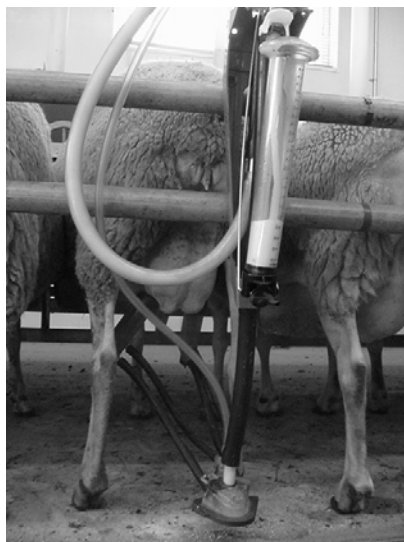
Picture 3. Meter jar installed in a high line pipeline on testing day
