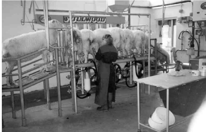
Picture 1. Permanently installed meter jars in a low line pipeline.
