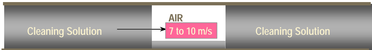
Figure 4. Principe of cleaning of a milkline in a milking machine.
