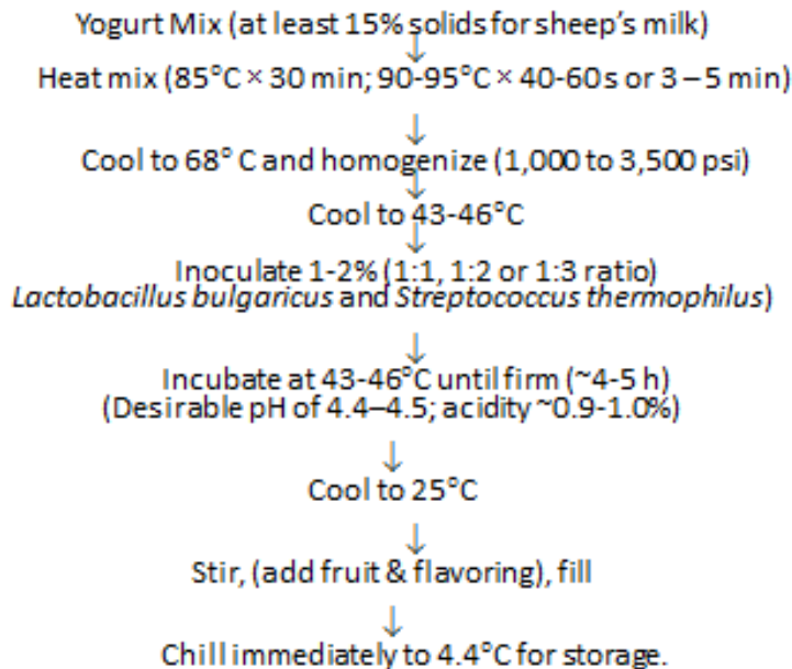
Figure 4. General manufacturing steps for stirred yogurt.
